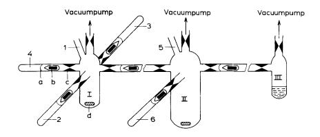
Figure I, fully closed apparatus for the synthesis of  $2.9-[^{14}C]$  dimethyl-1.10-phenanthroline.
